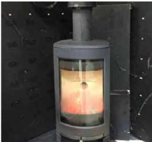
The stove on the test rig, output test
