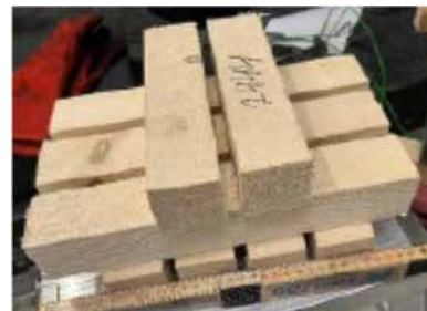
Placement of the fuel load in the firebox
